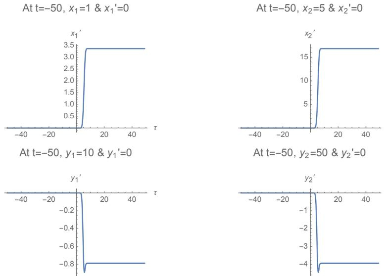
Figure 3.3: Velocity of the test masses at different times
