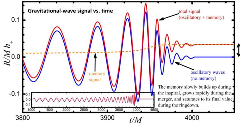
Figure 1.1: Memory effect on the strain data of the GW detector, Courtesy: M. Favata
